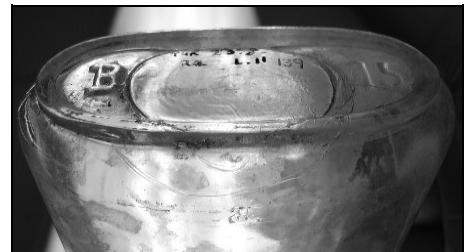
Figure 15 – Serif-B on heel and base – Owens machine
