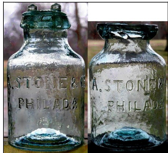
Figure C-22 – Lug finish – left; wax-sealer finish – right (North American Glass)
