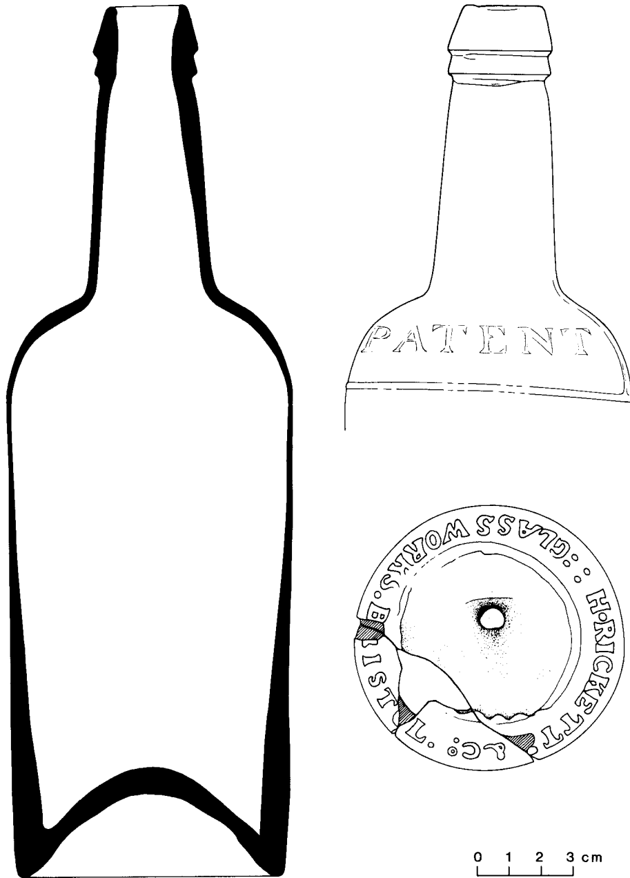
Figure 62. Bottle blown in the Ricketts' mould showing the characteristic mould lines of a "three-piece" mould in the body/shoulder area. The bottle is embossed on the base and shoulder. (Drawings by D. Kappler)
