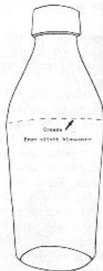
Figure 5. Bottles from a tapered dip mold will have no seams unless caused by a slight 'blow-over' at the base of the shoulder, or widest point. This is shown by the dotted lines.
