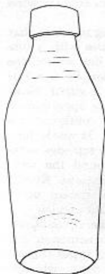
Figure 6. The turn-mold bottle will have no mold seams, but may have horizontal score-marks from an uneven mold surface.
