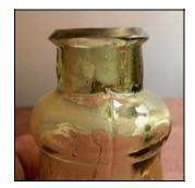
Figure 23 – Side seam on blacking bottle (eBay)
