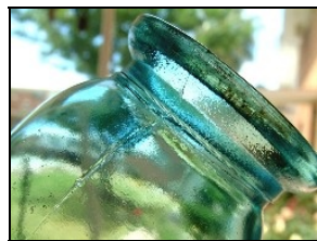
Figure 22 – Machine seams on wax-sealer finish
