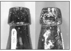
Figure 15 – A) one-part finish, tapered collar (San Elizario); B) one-part finish, rounded collar (San Elizario)
