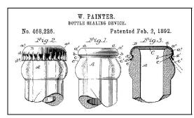
Figure 8 - Crown Finish - Painter 1892 Patent
