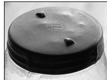
Figure 20 – Franklin jar lid with top projections and “bumps” in screw threads (North American Glass)
