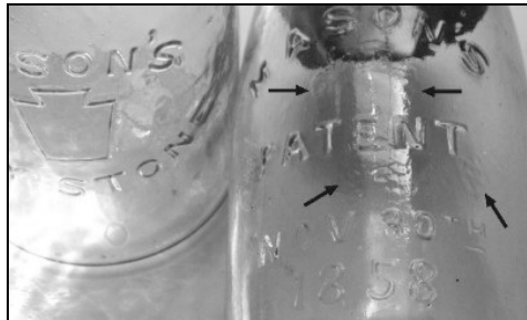
Figure 63 – Comparison of the Mason’s Keystone (left) and Mason’s Patent jar with ghosted keystone – arrows point to ghosted keystone emblem, letter “S” and letter “N” (Jim Sears collection)
