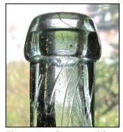
Figure 1 – Groove with squared bottom (eBay)
