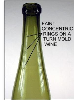
Figure 1 – Turn-Mold Bottle Characteristics (Lindsey 2014)
