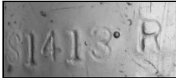
Figure 8-27 – Close-up of the “R” – note the right “leg” is thinner and shorter than the left one
