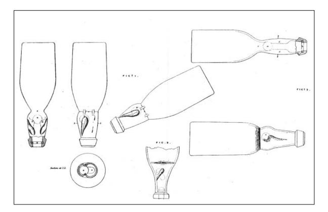
(Fig. 7) Original Codd bottle design
